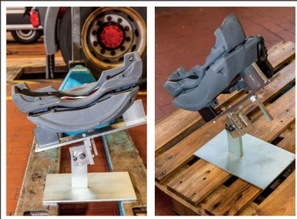
**NOTE!** 4972-2 Swivel bearing for disassembly and assembly of brake calliper in trucks, buses, trailers and trailer axles that are installed in a diagonal "clockwise position between 8 o'clock and 5 o'clock".
