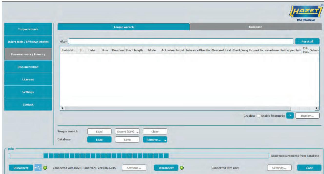
The measuring values at the wrench can be stored in the database. Switch into the database (top right tab) and "Load" the saved measuring values.
