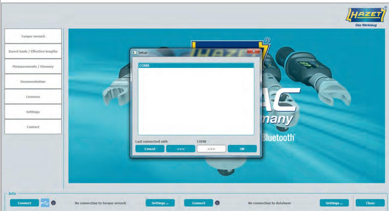
Select the corresponding USB port you want to use to connect to the HAZET SmartTAC torque wrench with built-in angle gauge.
