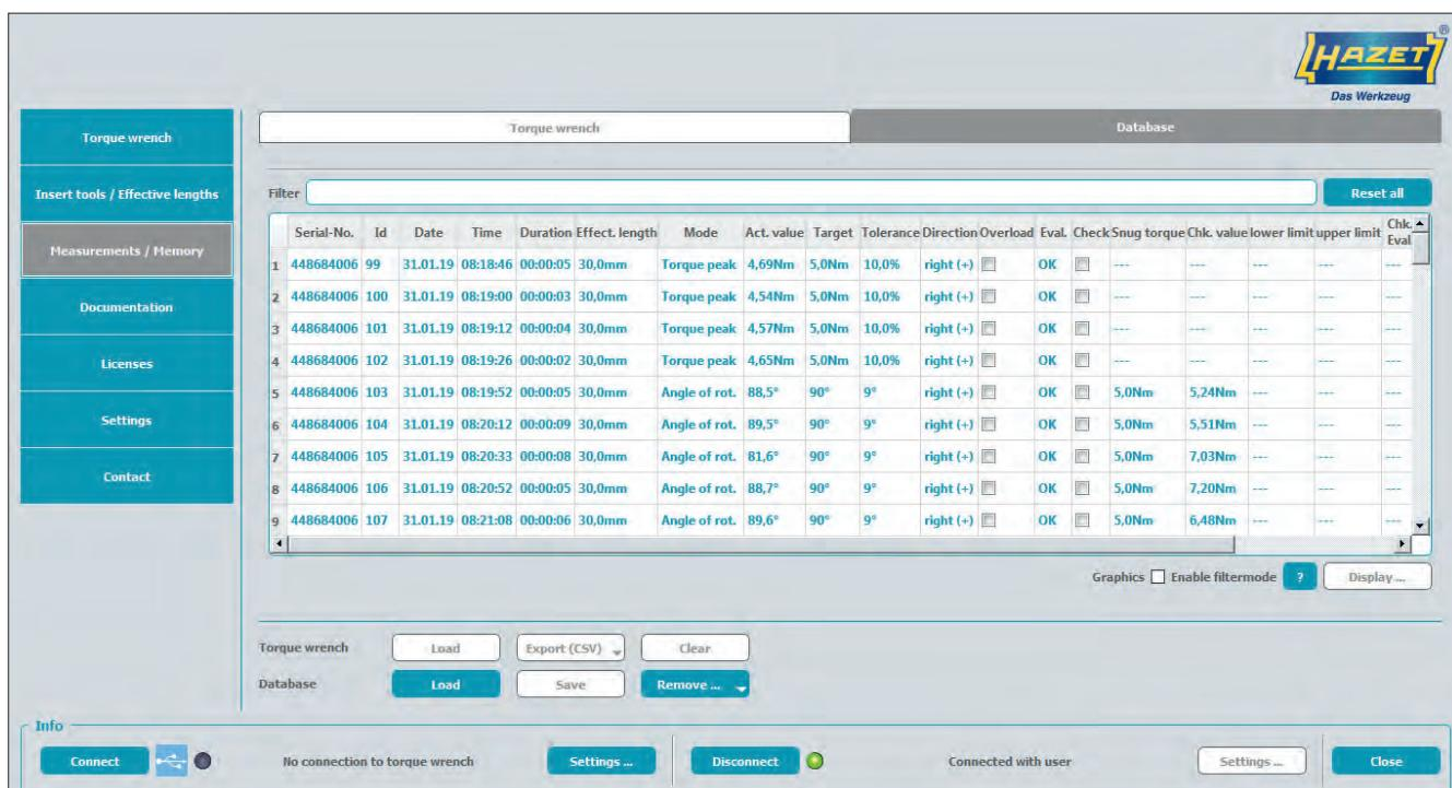
The torque wrench's measuring values are displayed in the database.
