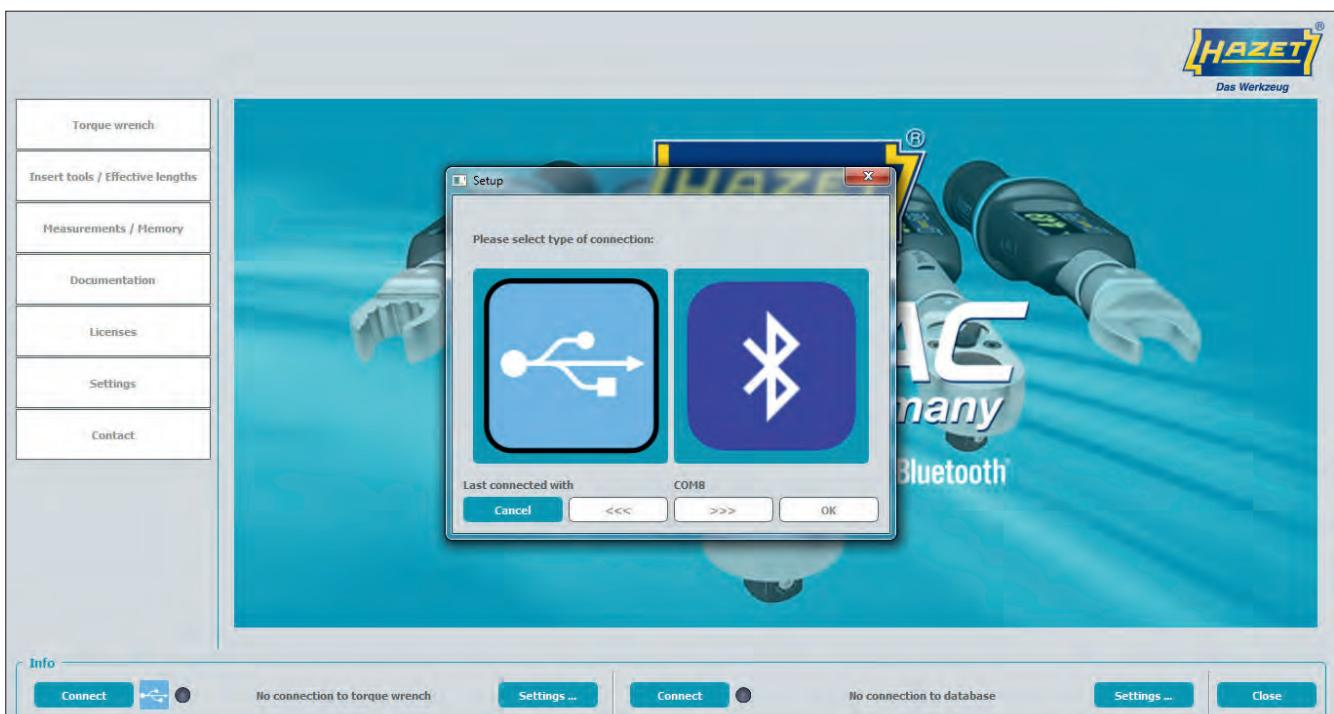
Launch the application. Before you can use the software, you must establish a connection to your HAZET SmartTAC torque wrench with built-in angle gauge. Select the connection type using the "Settings" button on the left-hand side to connect to your HAZET sTAC-wrench.
