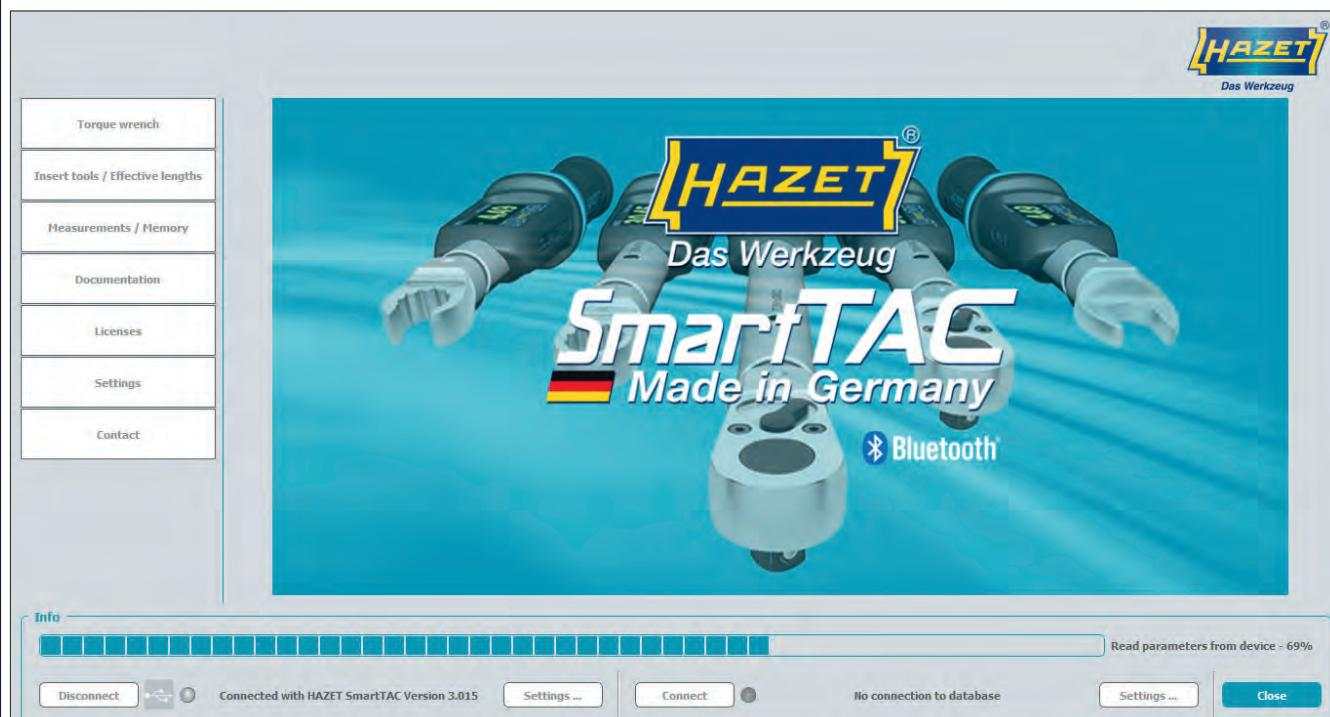
Once you have selected the port, connect your HAZET SmartTAC torque wrench with built-in angle gauge via the button on the left-hand side.
